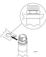
3. Align dots located on hose fitting, making sure they are facing each other at all times to ensure the hose does not twist during reinstallation.
